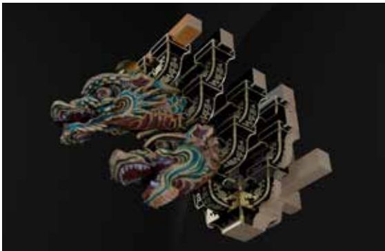
E. 東照宮陽明門組物模型(イメージCG) Toshogu Shrine, CG of a 3D model of Yomeimon Gate kumimono design
