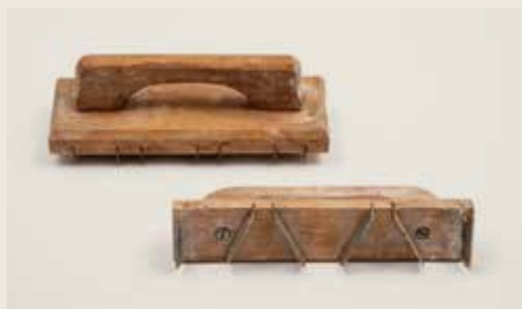
パリ滞時に用いたフランス製鋸ヤスリ French "chemin de fer" file used during stay in Paris
